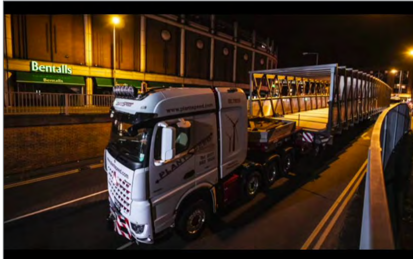
Figure 1-13: Example of Transportation of 4m Wide Prefabricated Pedestrian/Cycle Bridge Deck
