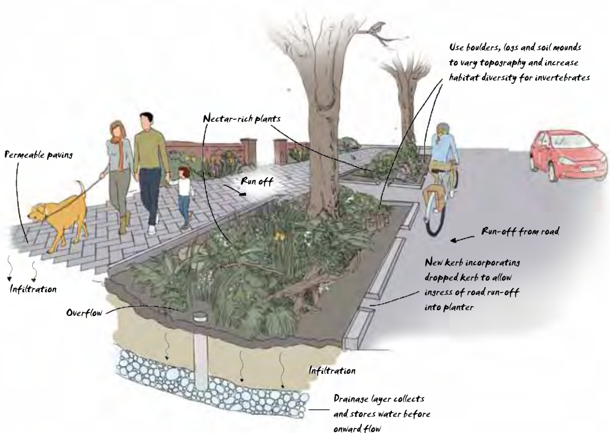
Figure 10 Bioretention areas enhance the streetscene, increase evaporative cooling and provide habitat for wildlife.
