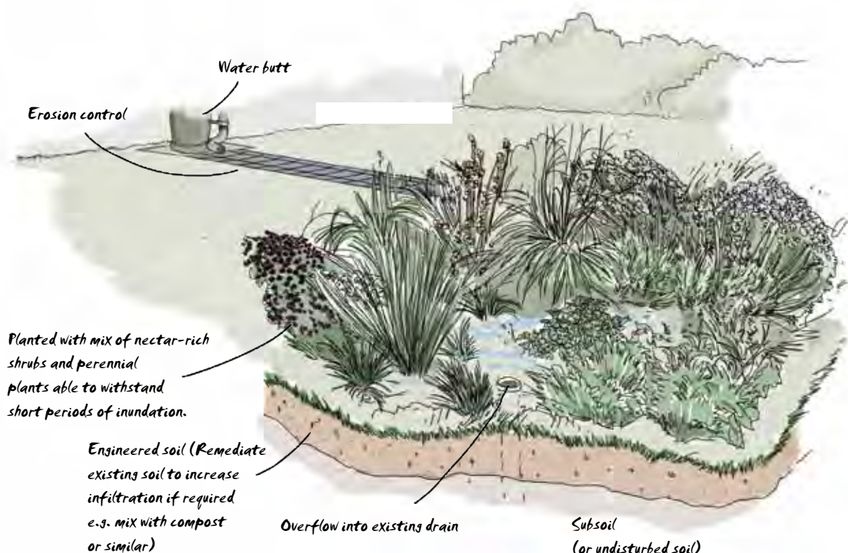
Figure 7 Rain gardens attenuate and clean surface water and provide valuable habitats in urban settings.
