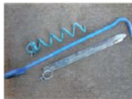
Two types of anchor: angle iron stake (below) and corkscrew (above). The man-hole cover lifter (centre) makes an excellent extraction tool for both anchors.
