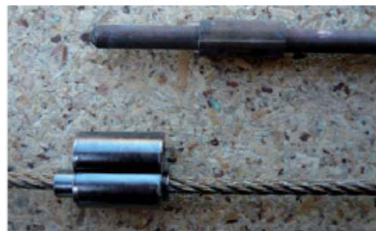
Copper wire tealer (top) and (below) the snare cable showing one style of tealer-clip. Note the collar on the tealer which prevents the clip sliding down.
