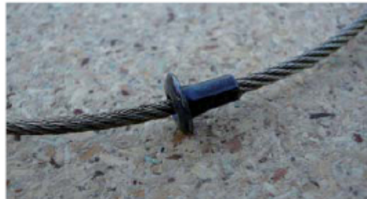
One kind of fixed stop, which prevents the noose closing too far
