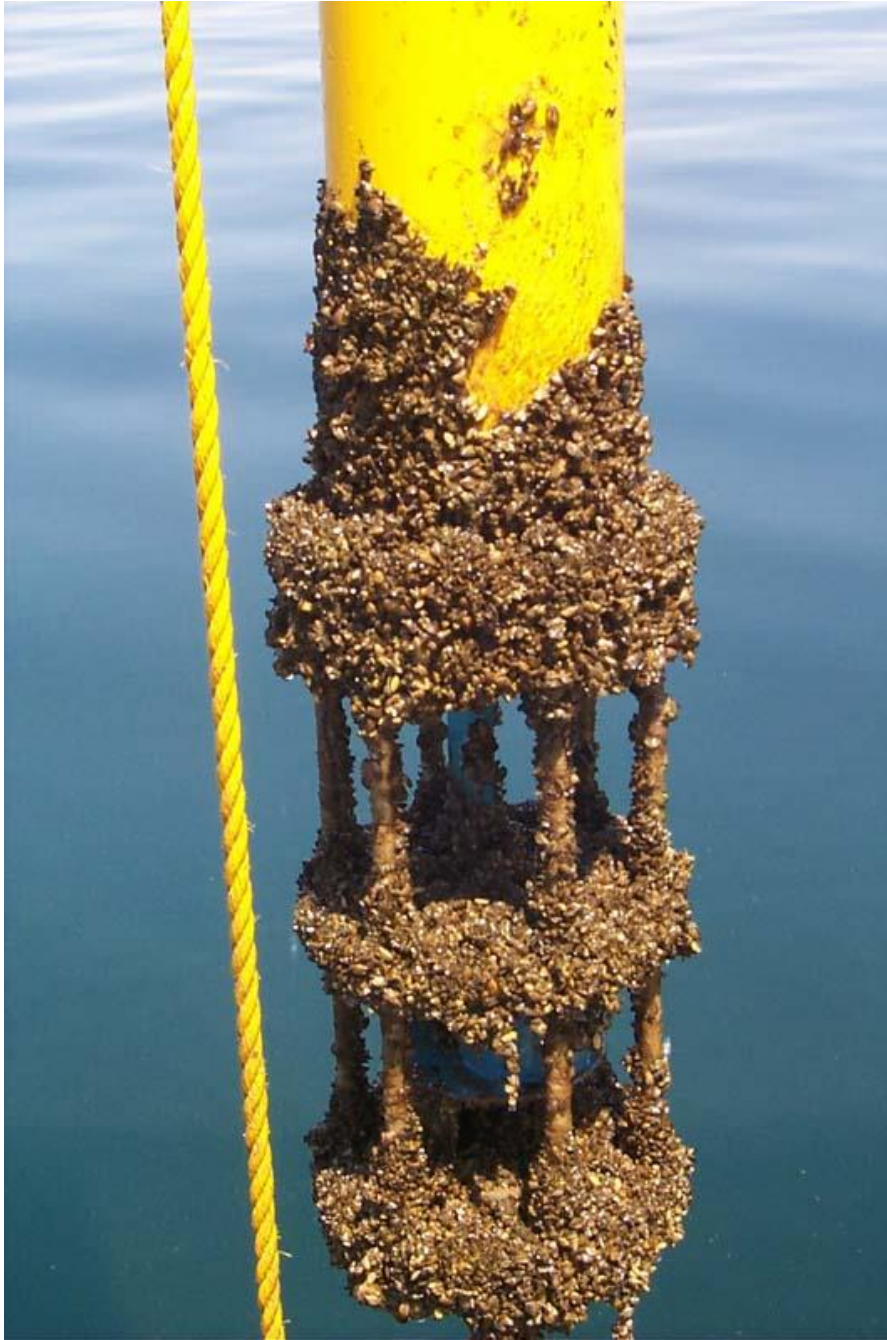
Figure 2. Zebra mussel-encrusted Vector Averaging Current Meter near Michigan City, IN. Lake Michigan, June 1999. NOAA, Great Lakes Environmental Research Laboratory. Image public domain, WikiMedia
