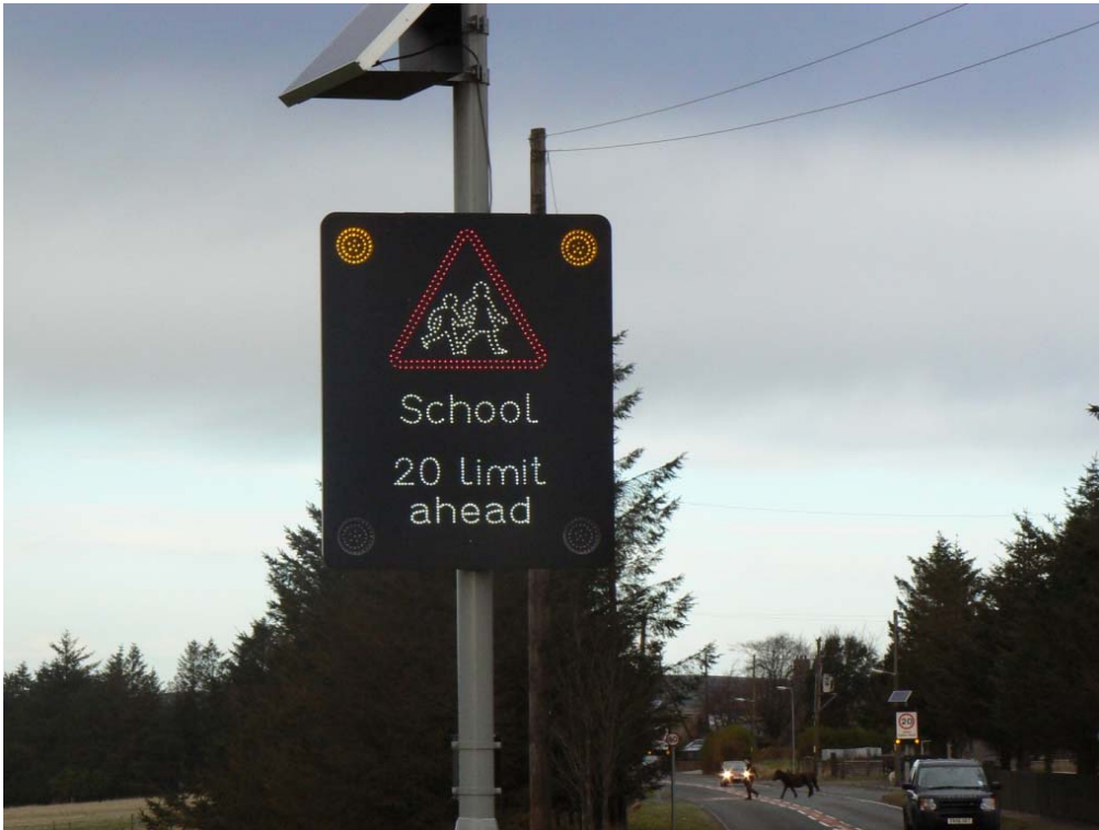
Rural solar powered Advance Slave Unit on local authority road (Aberdeenshire)
