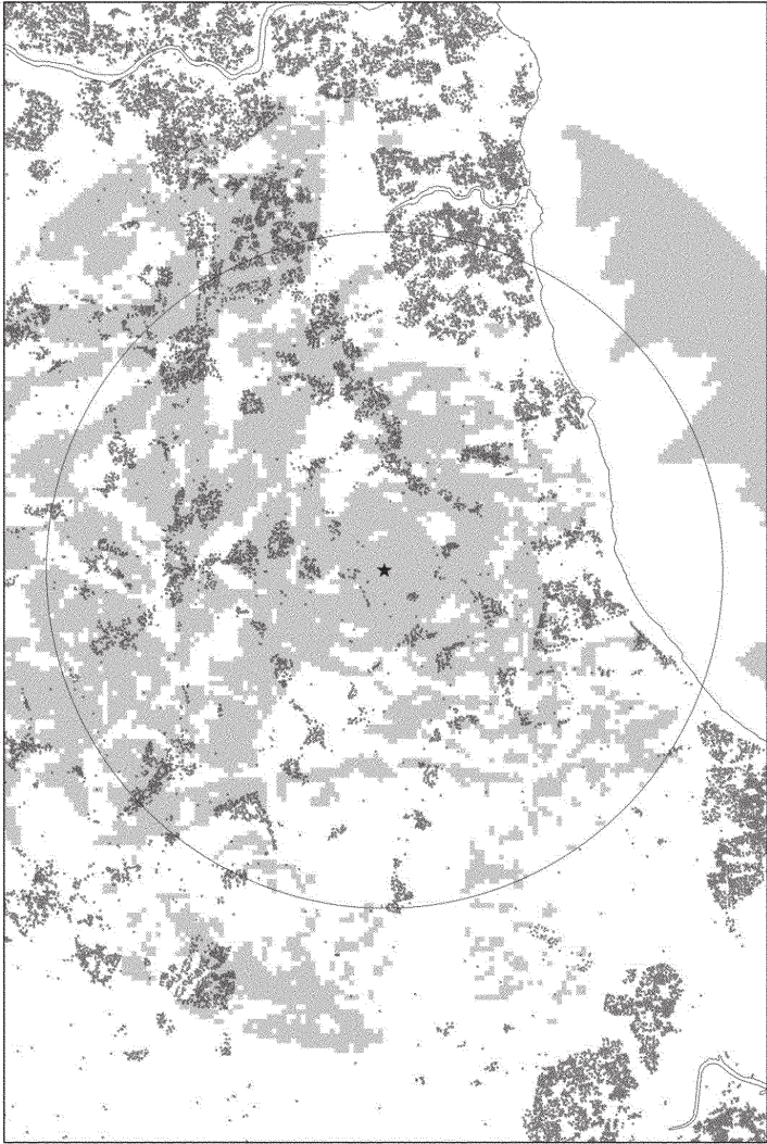
Figure 5: Example viewshed. Haswell Moor wind farm in north east England
