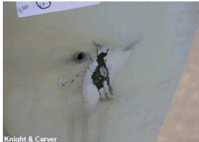
Figure 3 Wind turbine damage due to lightning strike
