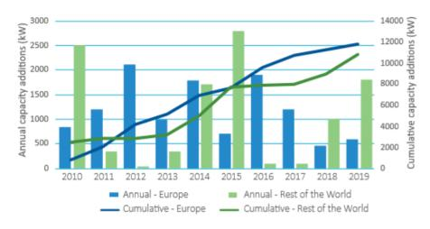
Figure 5: Annual and Cumulative wave capacity in European and the RoW 2010 to 201<sup>102</sup>9
