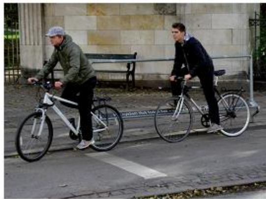
Figure 19 (Below): Foot rests at signalised intersections provide added comfort when cyclists do have to stop.
