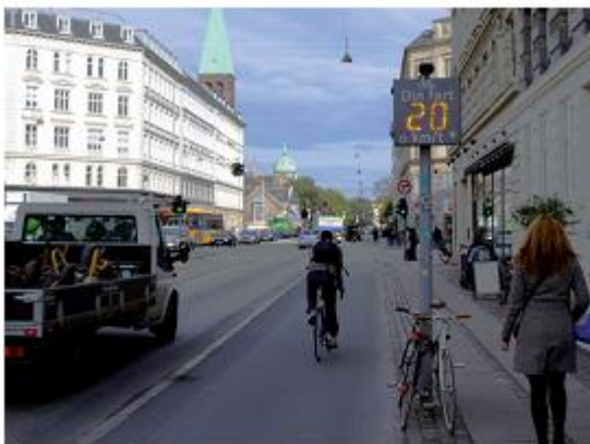
Figure 17 (Top left): “Your speed” counter helps cyclists maintain travel speed in the green wave.
