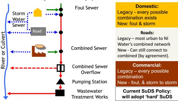
Figure 1: NI Water's sewerage system and duties<sup>32</sup>
