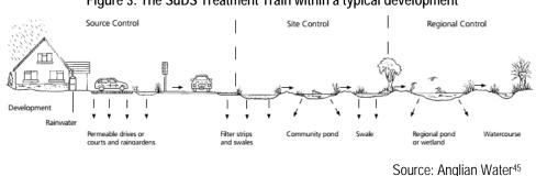
Figure 3: The SuDS Treatment Train within a typical development
