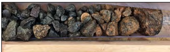
Fig.17 Washed out gravel in core 3.
